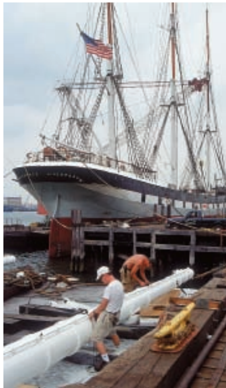
Volunteers attach rigging to completed steel yard at Caddell's Shipyard in Staten Island. Yards were designed by Charles DeRoko.
